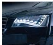
Covestro's high-transmission Makrolon LED2245 OC is found in headlamps as light guides and light pipes, and as a daytime running lamp.
