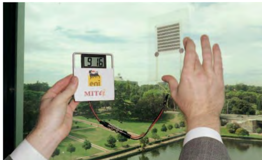
250 PV Cells = 50 Volts
