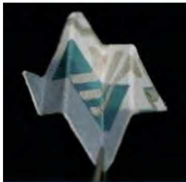
PV Cells Screen Printed on Newspaper
