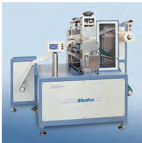
Lab-Scale Calendering Unit Courtesy Mathis AG
